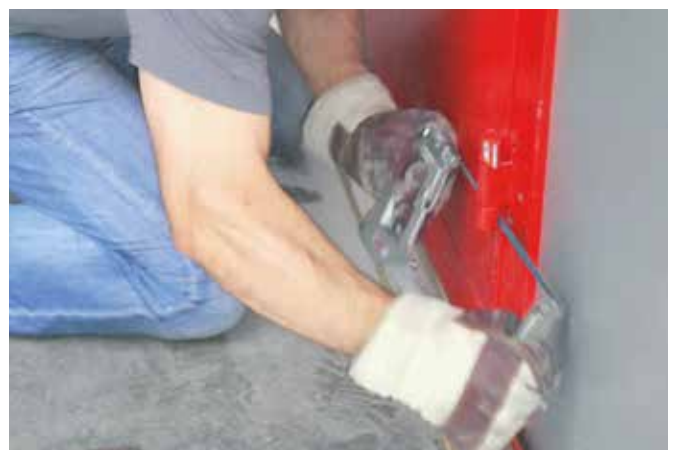
Break-in test: Attack on the hinges
