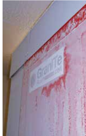
Test specimen after dust testing
